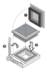
3 Attach one side of the fan/heatsink metal bracket to the CPU socket and then gently push down the other side of the metal bracket until it locks in place.
